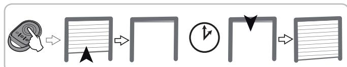
A new command during this time delay cancels automatic closing and the door remains open.
