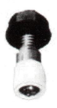
Standard roller guide for metal doors, used with either No. 10 or 12 Channel. Rustproofed steel spindles with nylon roller. Available with brass roller (not shown) specify No. 23B. No. 24 as No. 23 but with long spindle for R.H.S. Steel framed doors. No. 24B as No. 24 but with brass roller.
