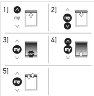
**2]** **To memorize the up limit:** Press the **My** and **Down** buttons simultaneously and release once the motorised product begins to move. The up limit is now memorized and green LED blinks 5 times.
