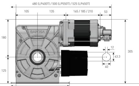
SIDONE, as standard, is for horizontal application. It can be installed in vertical position, according to the room available, by using the suitable basement.
